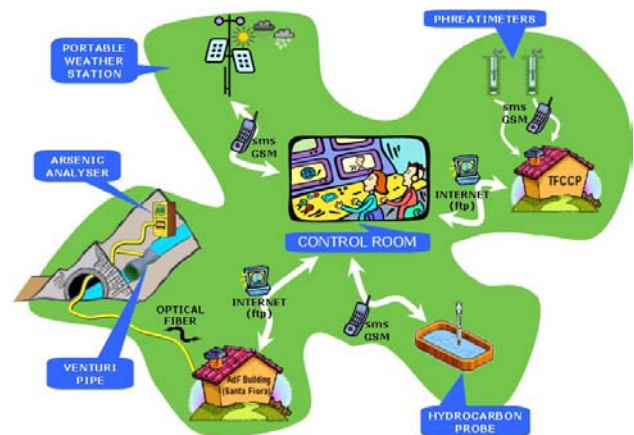
Figure 9. Sensor network architecture implemented in Santa Fiora for the OSIRIS water monitoring application.
