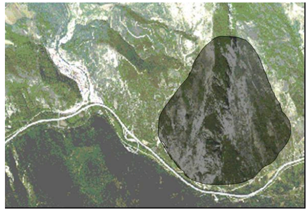
Figure 4. Identification of the vulnerable elements in the environment surrounding a major hazard industrial installation (railway, highway, urban and industrial settlements) and natural hazards (1965 landslide)
