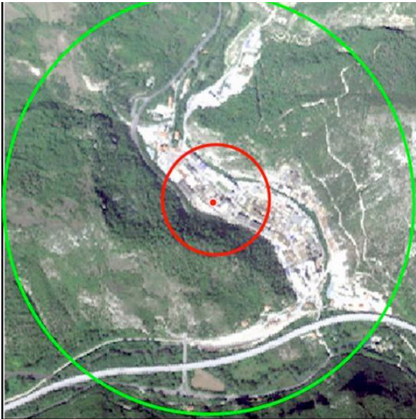
Figure 6. Visualization of the area of possible damage for Flash-fire (instantaneous thermal radiation): Zone I high lethality; Zone II lethality.
