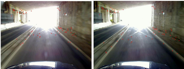
Figure 7: Example of extracted points in subsequent images in the tunnel test (4960-4961)
