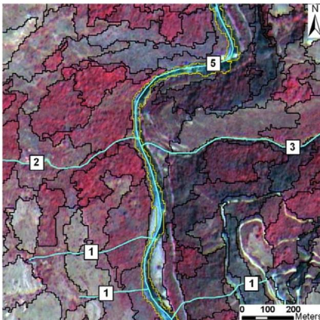
Figure 2. High order drainage (order 5 in this case) was used to classify objects as water body.
