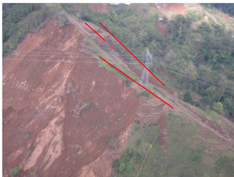
Fig.5. "NS" direction cracks. San Miguel-Cariblanco-Cinchona area
