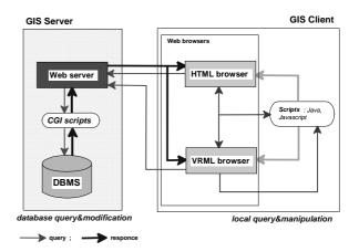
Figure 1: System architecture
