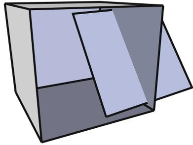
**Fig. 3** Geometric model for Fig. 1. A is a road surface ‘through’ the hole in solid building B. In this case the constraint ‘road A cannot cross building B’ is not violated
