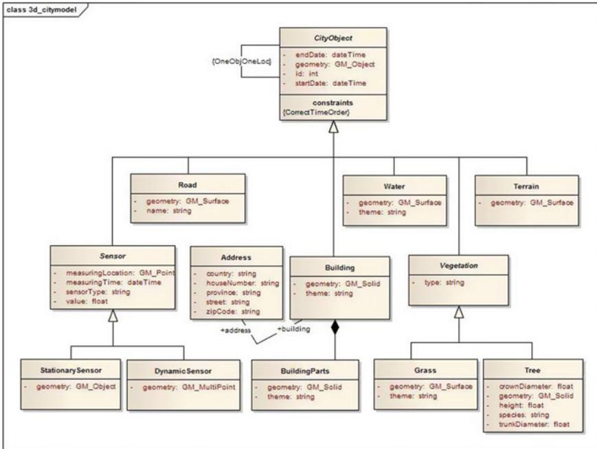
Fig. 4 UML model of constraints related to general city modelling (based on CityGML with extension on *sensor* class)
