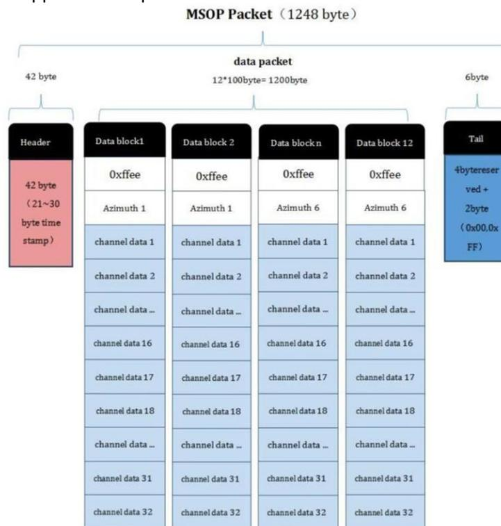
Figure 5: MSOP Packet structure
