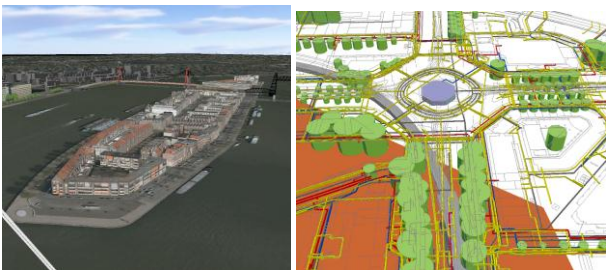
Fig 1: City of Rotterdam: 3D city model (left) and b) 3D underground infrastructure (right)
