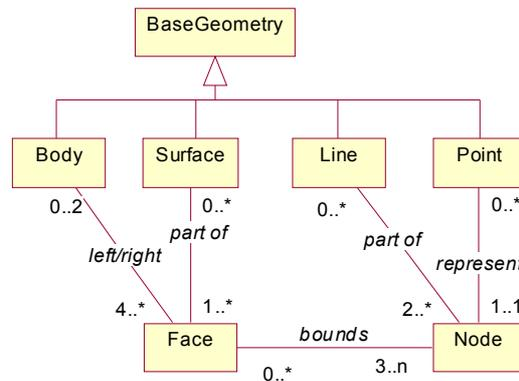
Figure 5: Geometry and topology in UDM
