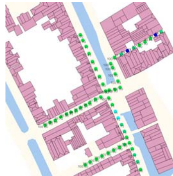
Figure 3: Combined Galileo and GPS: positioning in narrow streets is possible (only two dark dots remain undetermined)
