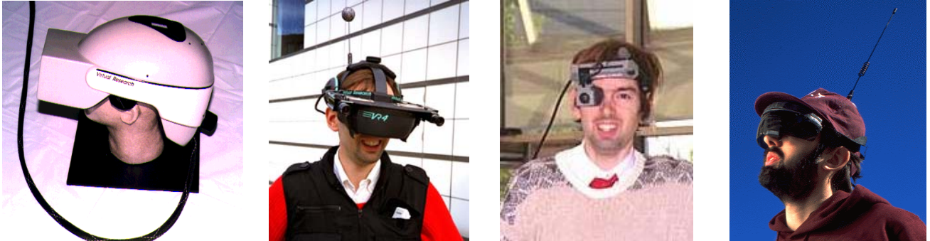
Figure 2-3: Displays: from completely isolated from real world view to see-through
